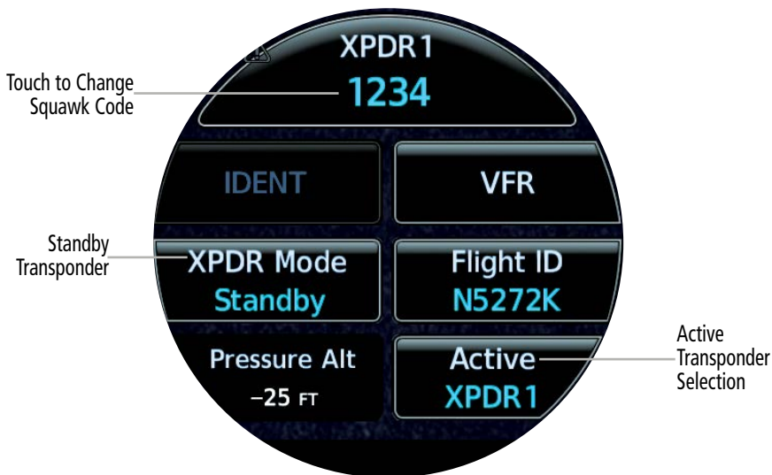
ADI - Transponder Control Display - Change Squawk Code
