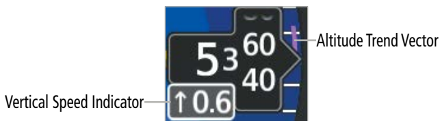
Vertical Speed Indicator and Altitude Trend Vector
