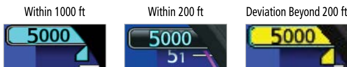
Altitude Alerting Visual Annunciations
