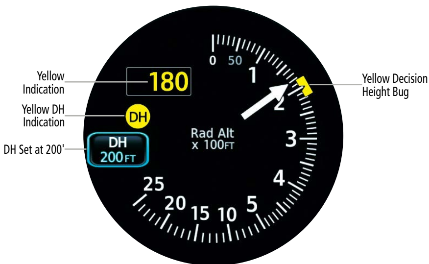
Airborne Indications - Below Decision Height - Fixed Wing
