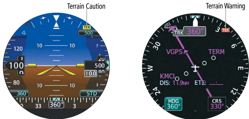
Primary ADI and Primary HSI Terrain Alert Examples
