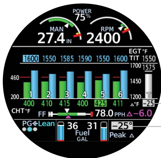
CHT/EGT - Lean Assist Alert Indication
